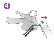
Put the needle of the gun through the material, close to the fold (a few mm away).
