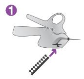
Insert fasteners into the Fixxon gun, using the bottom slot. Push until you feel them 'click' into place.
