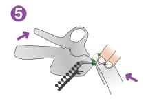
Whilst firmly holding the button and material against the gun, press the trigger to shoot the fastener through both button and material.
